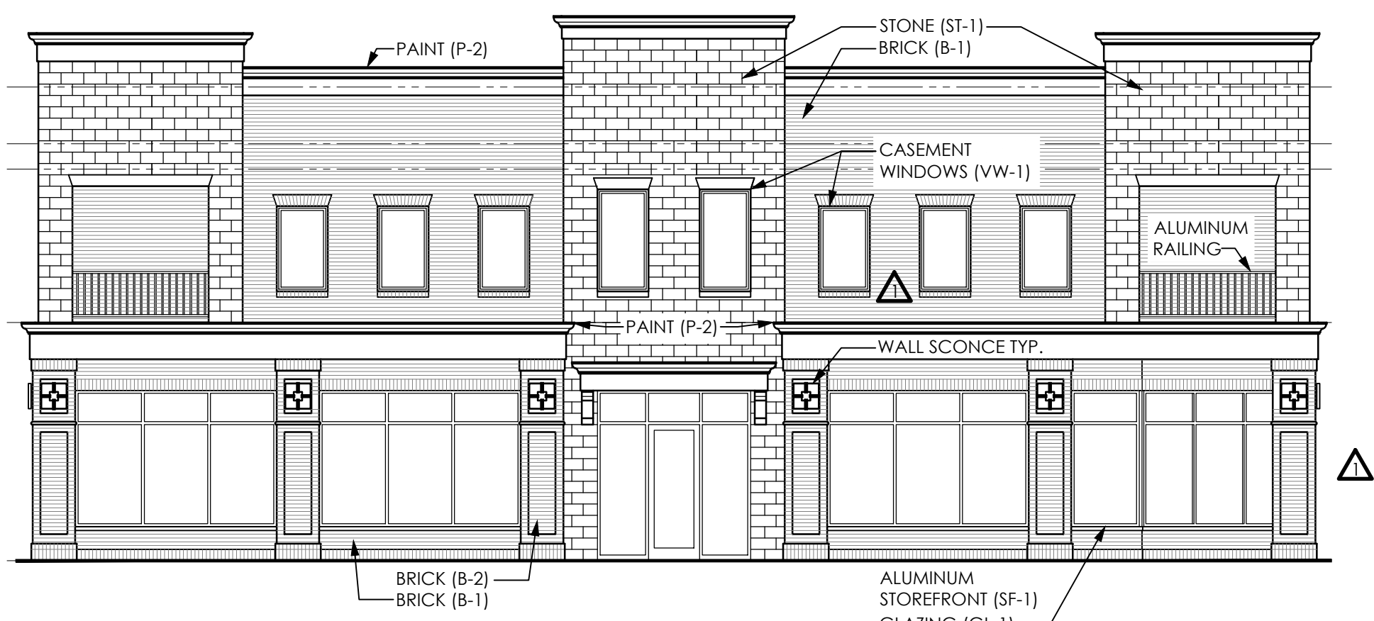
MILL STREET (EAST) ELEVATION SCALE: 1/8" = 1'-0"
